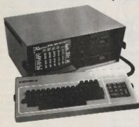
• Dual disk drives (400K capacity) • Interfaces for printer and communications • Detachable keyboard with numeric keypad • CP/M • Full complement of business applications software. See your local dealer for a complete demonstration.
